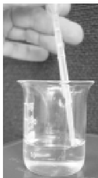
Figure 2 Limonene is isolated by pipetting the oil off the distillate.
